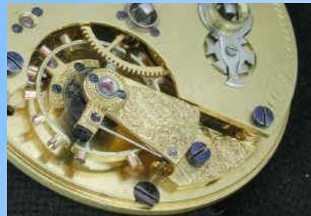
16KW, American Grade, with Stratton's barrel, exposed stop works, and Fogg's vibrating stud
