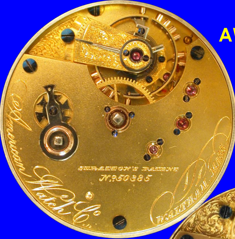
19J SN 50,385 Stratton's Barrel Lowest numbered run
