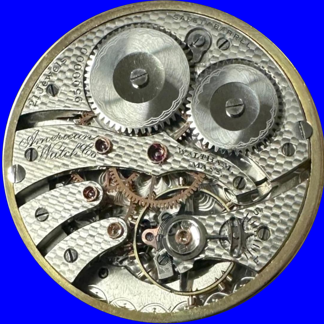
12 Size 1894 Open Face Model 9,500,000 21 Jewels, Gold Train & Jewel Settings Church's Patent Starwheel Regulator
