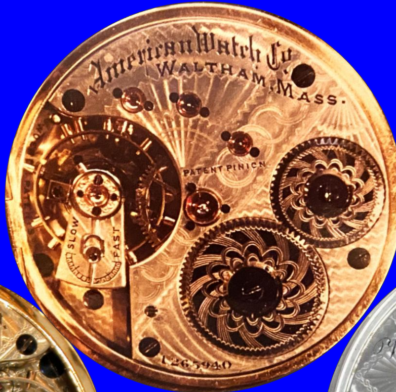
SN 1,265,940 Run #5 Unusual Plate DMK Possibly Unique Winding Wheels
