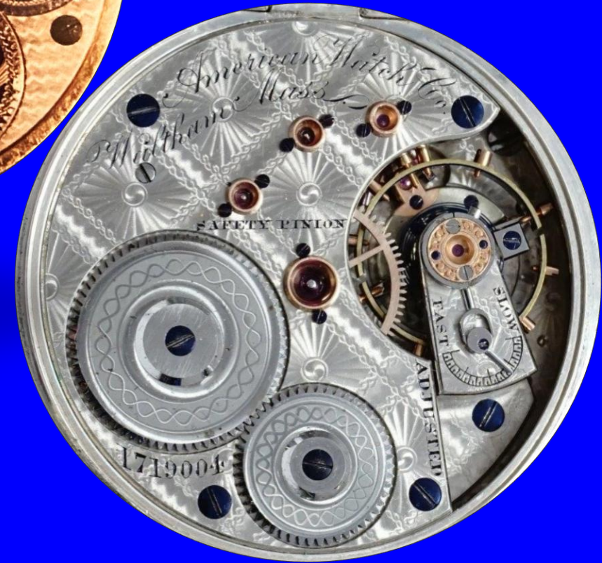
SN 1,719,004 Run #10 Only Gold Dome Run w. All raised Jewel settings on Top Plate (Courtesy, Jones & Horan)
