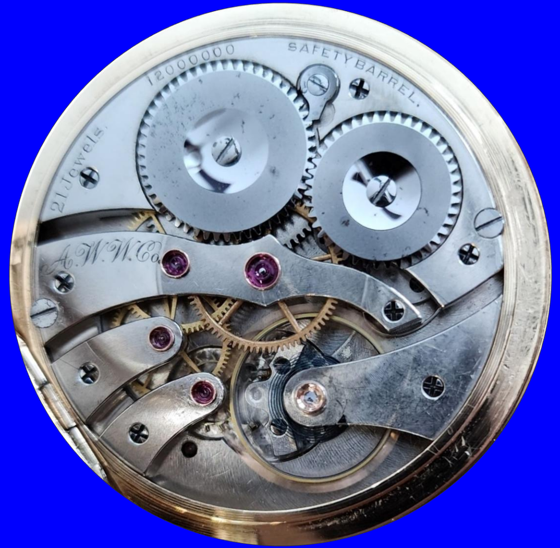
12 Size 1894 Open Face Model SN 12,000,000 21 jewels, Gold Train & Jewel Settings, Freesprung w. Coles Resilient Banking Escapement
