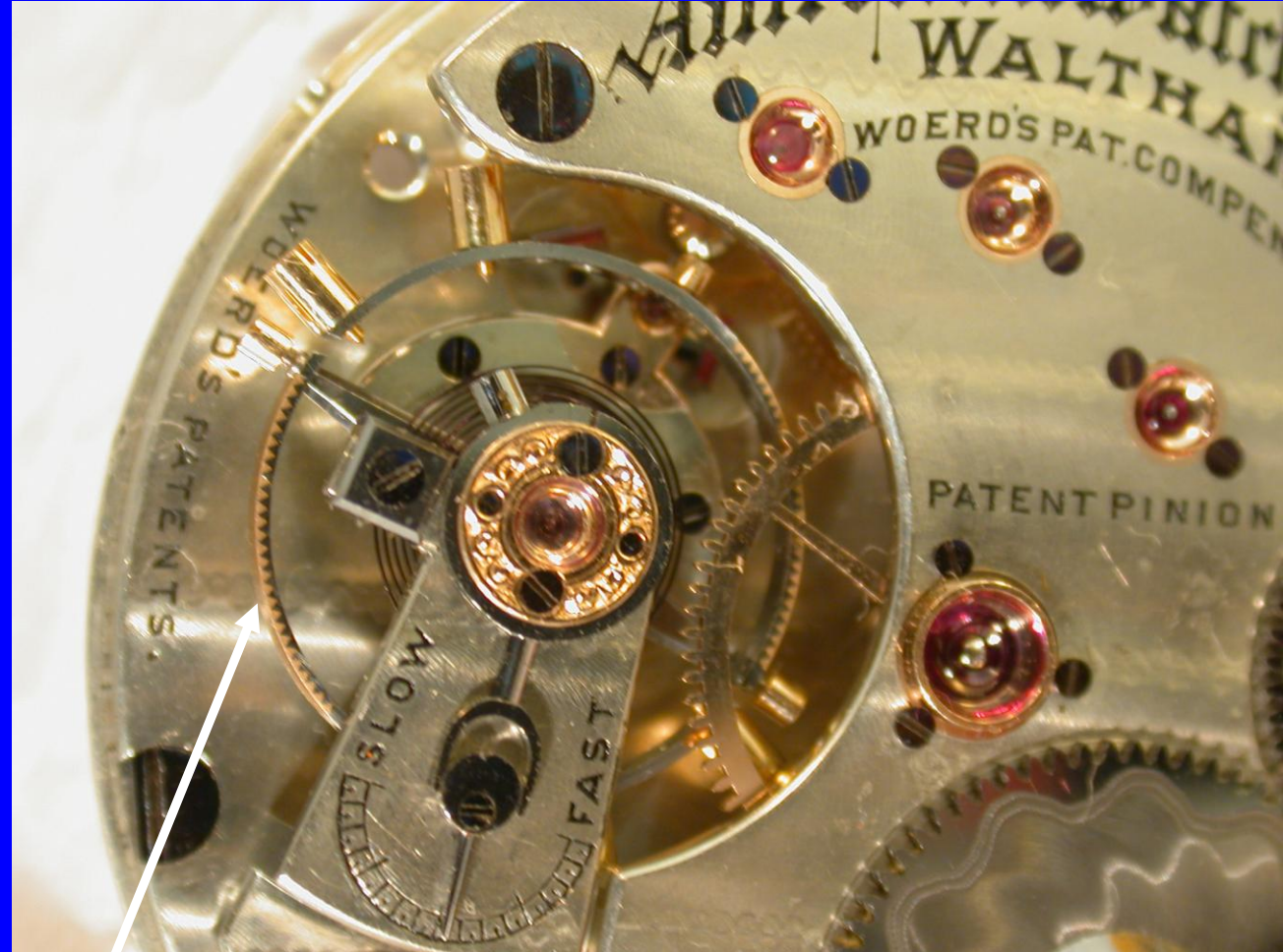
Woerd's Patent Compensating Sawtooth Balance (intended to reduce Middle Temperature Error)
