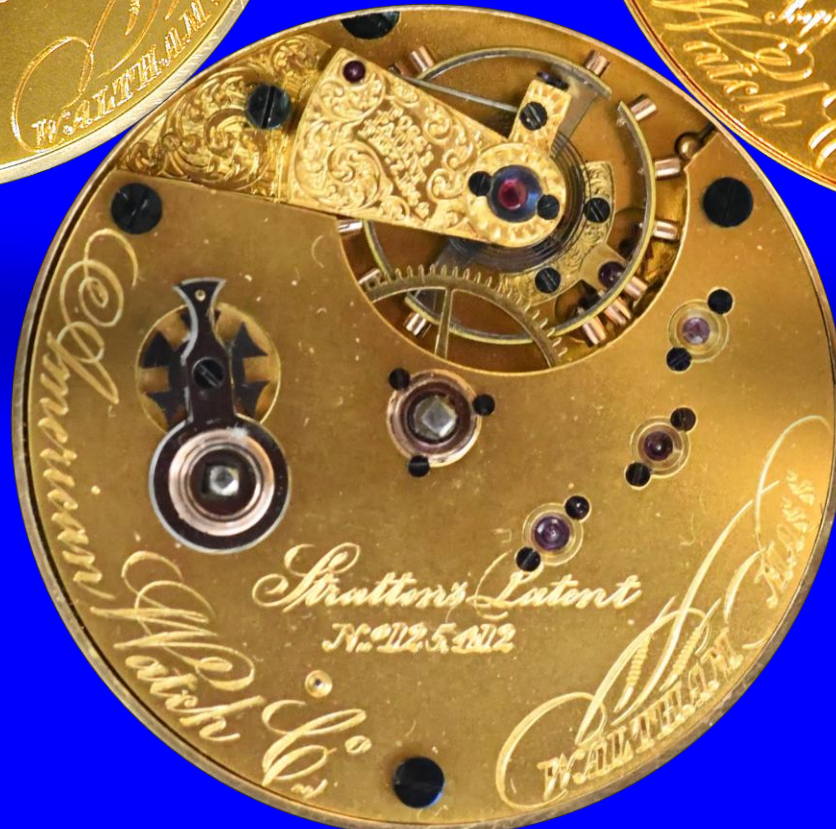
20J SN 125,412 Stratton's Barrel Fogg's Vib. Reg.
